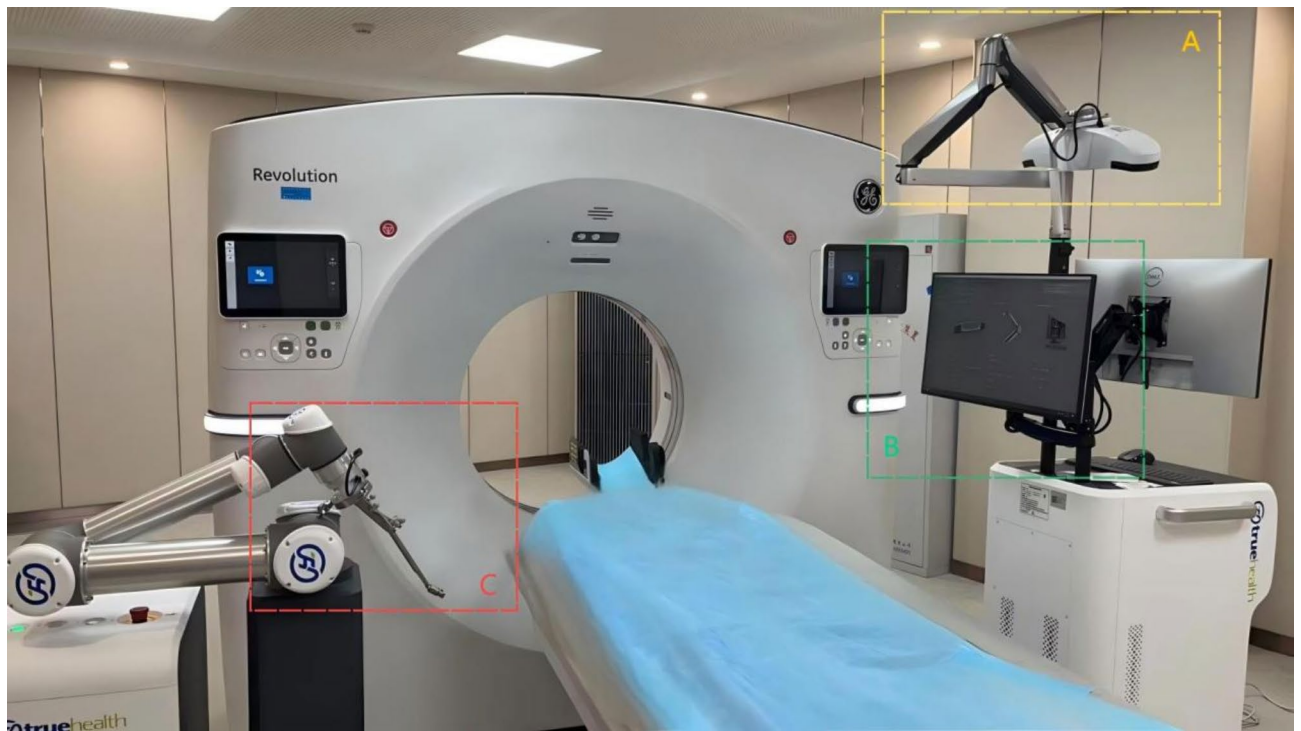
Fig. 1. The robotic-assisted navigation system. (A) The photoelectric navigation system used to track the position of the robotic arm and the patient; (B) the surgical planning system employed for the precise planning of the needle insertion path; (C) the robotic arm positioning and puncture system responsible for accurate positioning of the needle holder and assisting with needle insertion.
