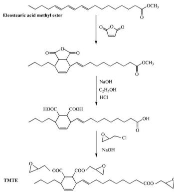
Figure 4. Synthesis of tung-maleic triglycidyl esters (TMTE).
