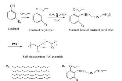
**Figure 25.** Synthesis of self-plasticization PVC via substitution reaction with minnich base of cardanol butyl ether.
