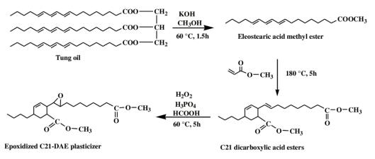
Figure 21. Synthesis of C21 dicarboxylic acid ester.
