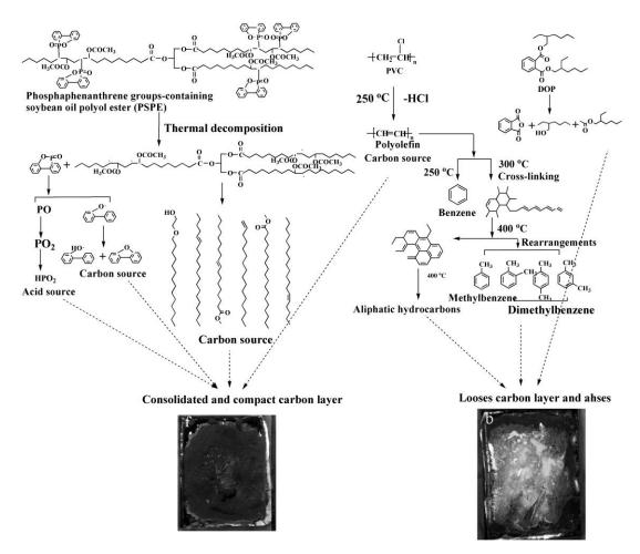
Figure 15. Flame retardant mechanism of DOPO groups-containing soybean oil polyol ester.
