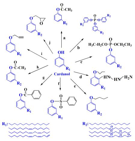
Figure 5. Chemical structure of cardanol based plasticizer.
