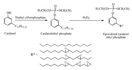
Figure 11. Synthesis of epoxidized cardanol ethyl phosphate.
