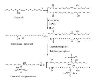
Figure 12. Synthesis of castor oil phosphate ester.
