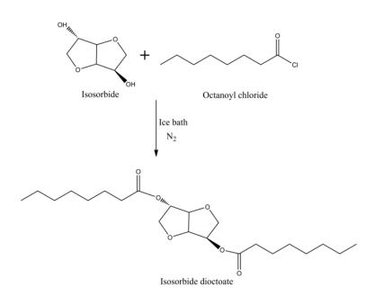
Figure 20. Synthesis of isosorbide dioctoate.
