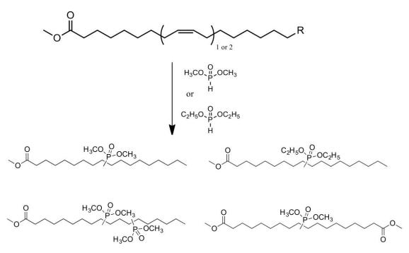
Figure 18. Synthesis of phosphonate groups containing bio-based plasticizers.
