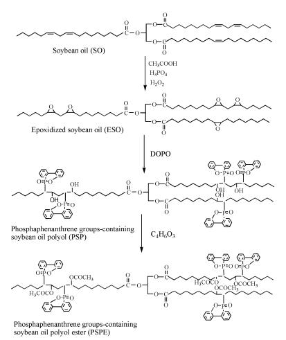
Figure 14. Synthesis of DOPO groups-containing soybean oil polyol ester.
