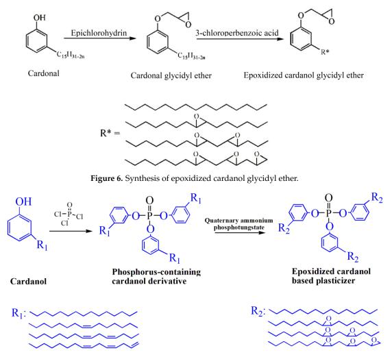
Figure 7. Synthesis routes of epoxidized cardanol based plasticizer (ECP).
