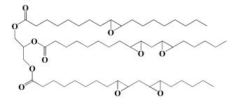
Figure 1. Chemical structure of epoxidized soybean oil.
