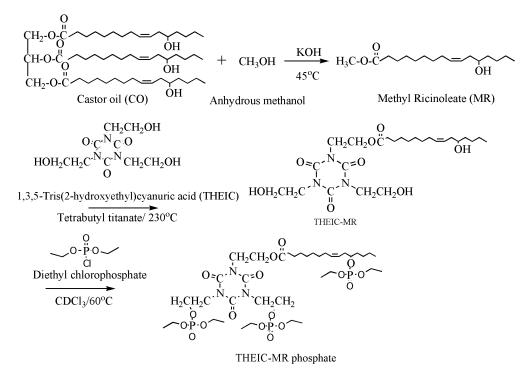
Figure 16. Synthesis of THEIC-MA phosphate.
