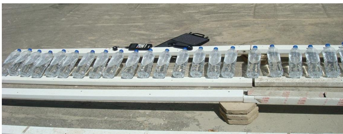
Fig. 2: SODIS reactor configuration
