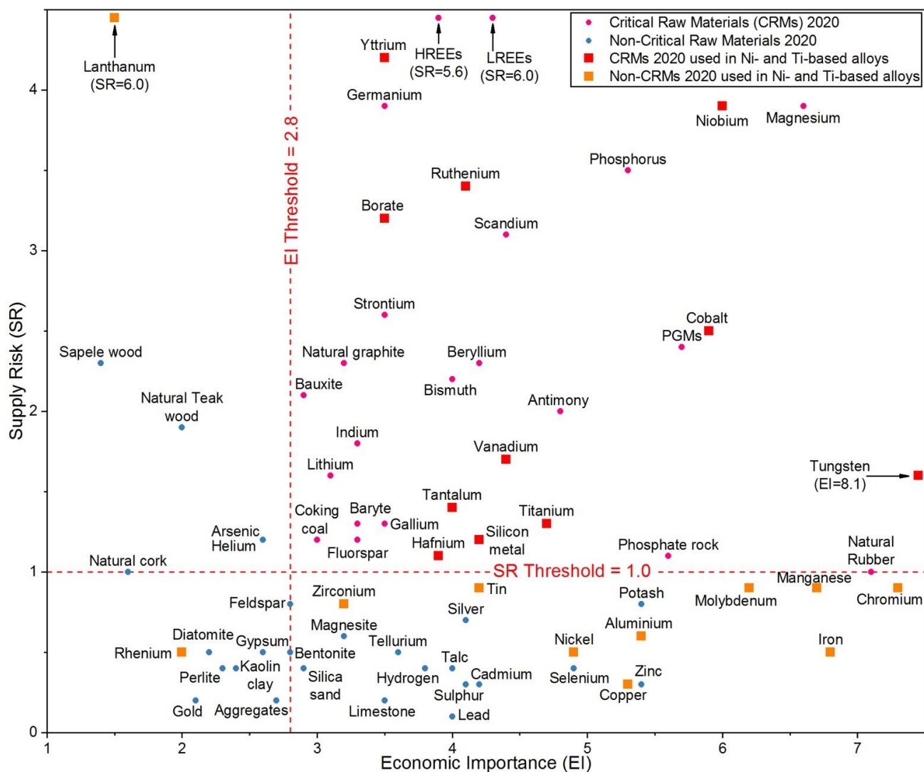
Figure 1. CRMs in 2020 for the EU (adapted from Ref. [3]). LREEs and HREEs stand for light and heavy rare earth elements (REEs), respectively.
