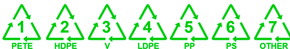
Figure 8. Designations for different groups of plastics in recycling according to [81].
