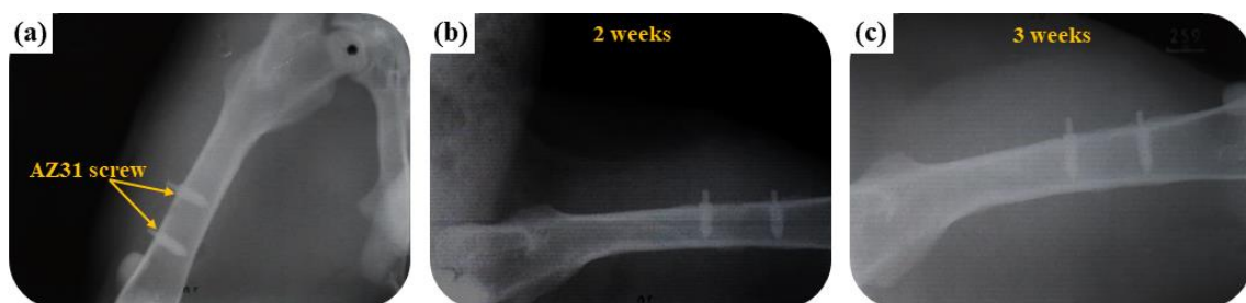
Figure 11. Plain X-ray of the AZ31 screw treated in the EDTA 7.5 g bath in the femoral shaft of a rabbit: (a) just implanted, (b) 2 weeks, and (c) 3 weeks.
