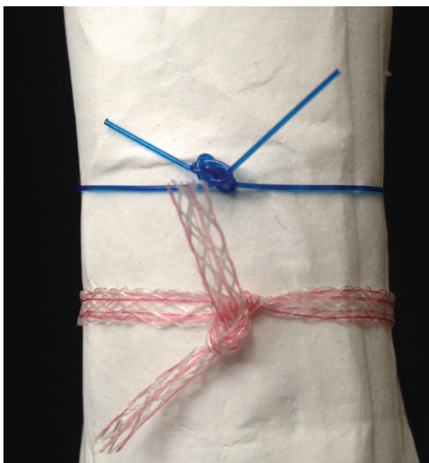
Fig. 3 0-Polypropylene and mesh suture below encircling an object, with representative knots. The mesh suture assumes a ribbon shape owing to lateral contact
