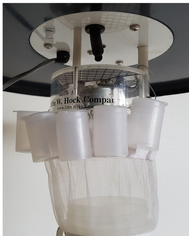
Fig. 1 Placement of vials releasing odor compounds on the CDC light trap
