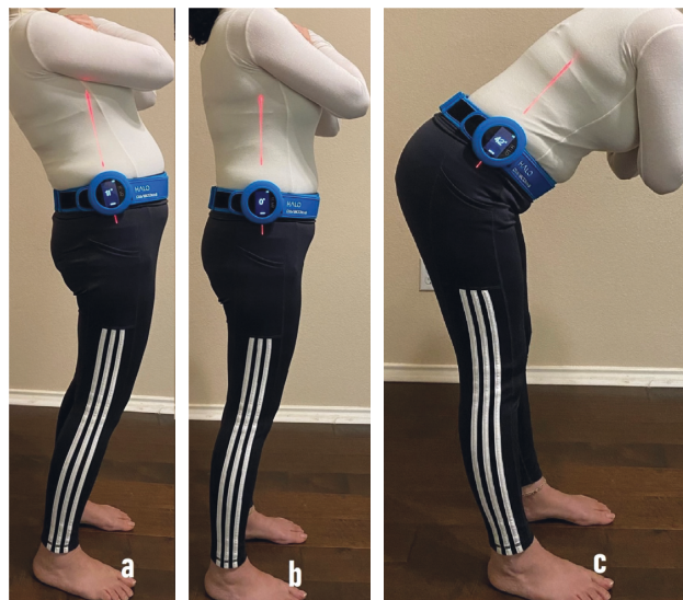
FIGURE 2: Measurement of the (a) trunk extension, (b) neutral, and (c) trunk flexion. A laser-guided digital goniometer (HALO) is fastened to a belt around the waist while standing.
