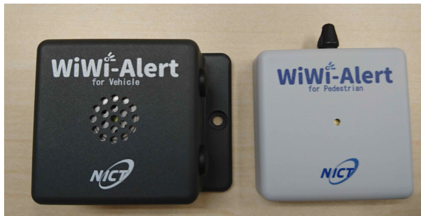
Figure 7. The prototype devices for a vehicle ( left ) and a pedestrian ( right ). The size of both devices is 5\text{ cm} \times 5\text{ cm}
