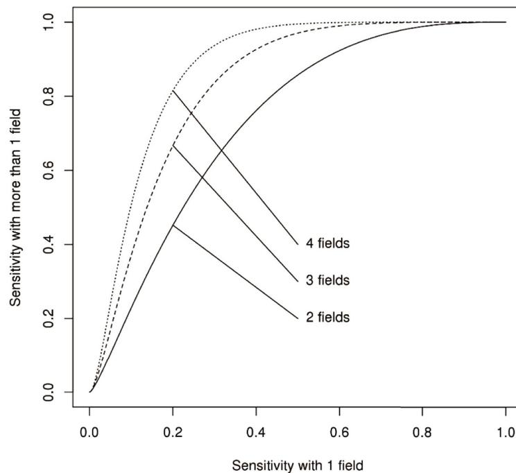
**Fig 4. Assay sensitivity comparisons.** The improvement in sensitivity that is possible by using multiple fields.
