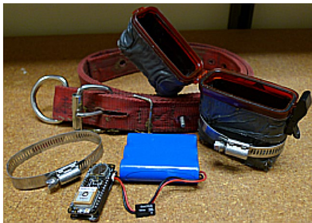
FIGURE 1 Top: Illustration of our Global Positioning Systems (GPS) datalogger electronics. Basic components include the Adafruit Feather M0 Adalogger (a) and Adafruit GPS Wing (b). Also shown are the TPL5110 low power timer (c), external JST battery plug (d), and a 47uF capacitor (e) to stabilize the power supply. Bottom: The assembled GPS Wing and Adalogger, with battery, case, clamps, and collar
