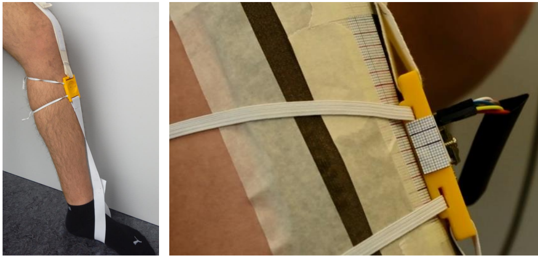
Figure 8. Measurement setup to assess sensor functionality during unloaded knee bends: sensor platform with elastic attachment ( left ) and integration of quantification method ( right ).
