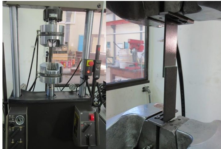
Figure 6. Test set-up for the tensile shear fatigue test with a single lap shear FM® 300K specimen clamped in an MTS 810 servo hydraulic testing machine with a 100 kN load cell at the University of Patras (Greece).
