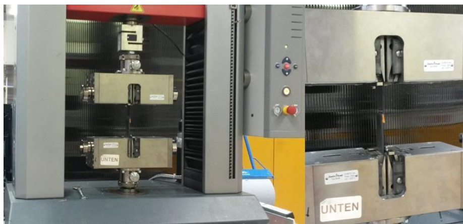
Figure 3. Test set-up for the quasi-static tensile shear test with a single lab shear FM® 300-2K specimen clamped in a Z020 ZwickRoell universal testing machine with a 20 kN load cell at Fraunhofer IFAM (Bremen, Germany).
