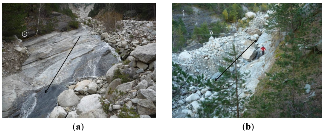
Figure 1. Factors affecting the ground vibration signal: characteristics of transmission medium between geophone and flow path. The transmission medium can be bedrock (a) or colluvium (b). The location of geophones is indicated by a circle; while the flow direction, is expressed by an arrow.
