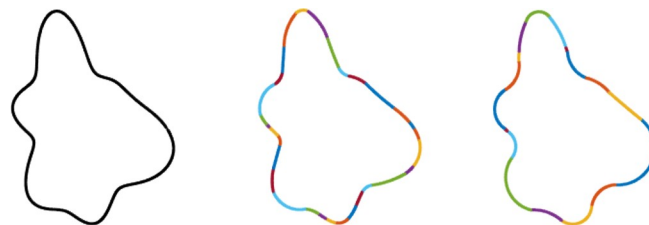
Fig 5. Two constant curvature representations of a shape contour. The original shape (left) is approximated with a small W (middle) and a large W (right). The smaller integration window has more segments and is more precise, organizing regions of the original shape with less variance in curvature into a single constant curvature segment (mean standard deviation of curvature = 0.02 per segment), while the larger integration window has fewer segments, but represents the contour less precisely, organizing regions with more curvature variance into single constant curvature segments (mean standard deviation of curvature = .05 per segment).
