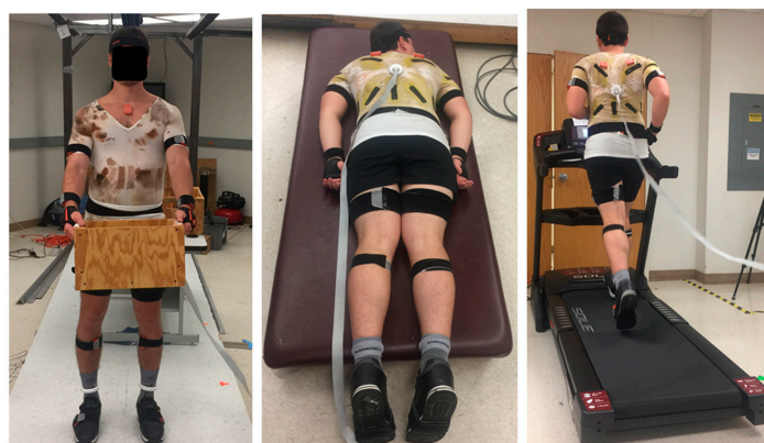
Figure 1. Illustrations of a participant wearing two smart textile systems (STs) (an SUS and smart socks) and a full-body inertial measurement unit (IMU) system during a sample of activities: carrying a box ( left ), laying down ( middle ), and running on a treadmill ( right ).
