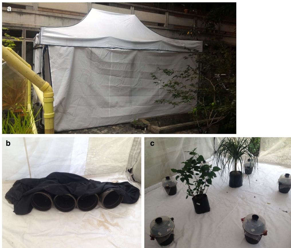
Fig. 2 Set-up of the semi-field cage. a Field cage exterior. b Field cage interior, showing close-up view of buckets with cloth. c Field cage interior, showing placement of ovitraps and resting sites: buckets with cloth and plants
