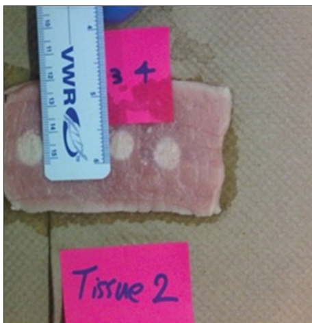
Figure 3: Tissue samples showing the length of the high-intensity focused ultrasound lesions (tissue #2, lesion #4)
