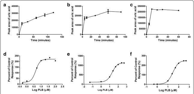
**Fig. 2** Confirmation of optimal incubation conditions. **A, B, C** Variations in the production of uric acid over time in MLS9, HLS9 and XO, respectively. Each point and error bar represents the average and S.D. of duplicate measurements. **D, E, F** The EC<sub>50</sub> values of PLB in MLS9, HLS9 and XO for the activation of XO. Each point represents the average of duplicate measurements
