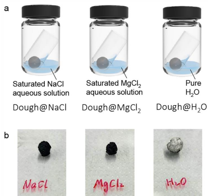
Supplementary Figure 23. a) MXene doughs were hermetically stored in the vials with different water vapor pressure. b) The photos of MXene dough after stored for 6 months at above environments.
