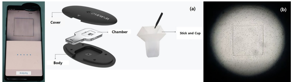
Fig 1. Installed OviewM and View of Sperm analysis using Oview M. (a) Consist of Oview M (b) View of Sperm analysis using Oview M.
