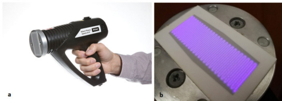
Figure 1. The photos are illustrating RPS40 plasma system, the general view of the handheld device (a) and the view of the macroscopically homogeneous DCSBD plasma layer generated in ambient air (b).
