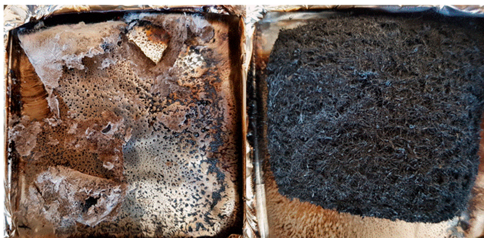
Figure 7. Residues from cone calorimeter for untreated wood fibers (left) and wood fibers with FR weipro (right).
