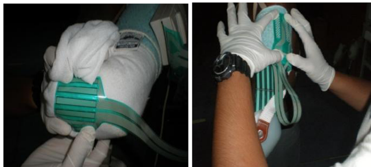
Figure 6 The F-socket sensor attach to the subject residual limb.
