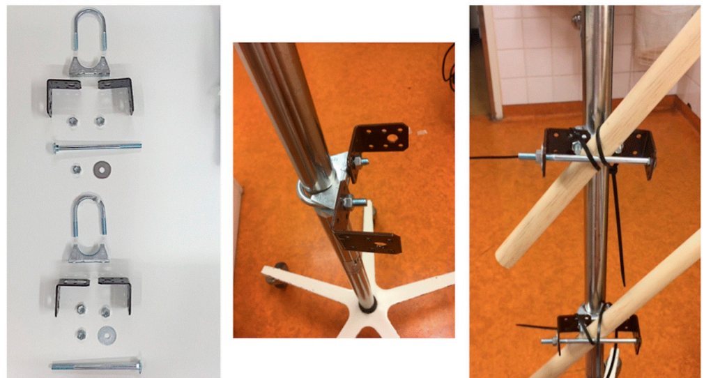
Figure 2. Construction of Tilted modality. Photo by author.
