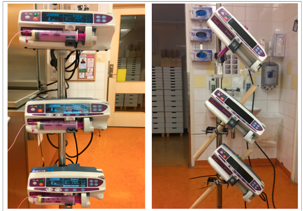
Figure 1. Horizontal and Tilted Pump Set Up. Photo by author.
