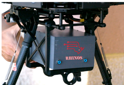
Figure 5. Integration of the RHINOS e-nose underneath the DJI Matrice M600 drone using a custom payload bay
