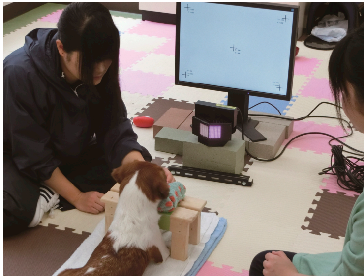
Figure 1. Subject dogs lied down in front of an eye-tracking camera and display. During calibration and the experimental session, the subject put his/her jaws on a purpose-designed chin rest.
