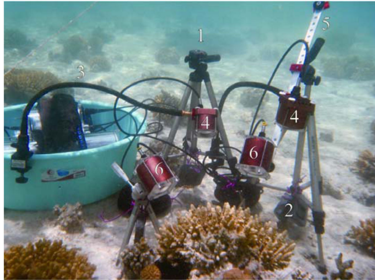
Figure 4. Symbolic underwater image of the video system. Tripods with a 3-way-pan-tilt head (1) and fixed diving weights (2) provide a stable and easy setup of cameras under water, while gooseneck stands (3) orientate the infrared-lights (4). To facilitate alignment of camera distances and for recordings in bird's eye view, flat aluminum bars (approx. 50 \times 1 \times 0.5 cm) perforated with 1/4'' holes (5) are used as extensions between cameras (6) and tripods.
