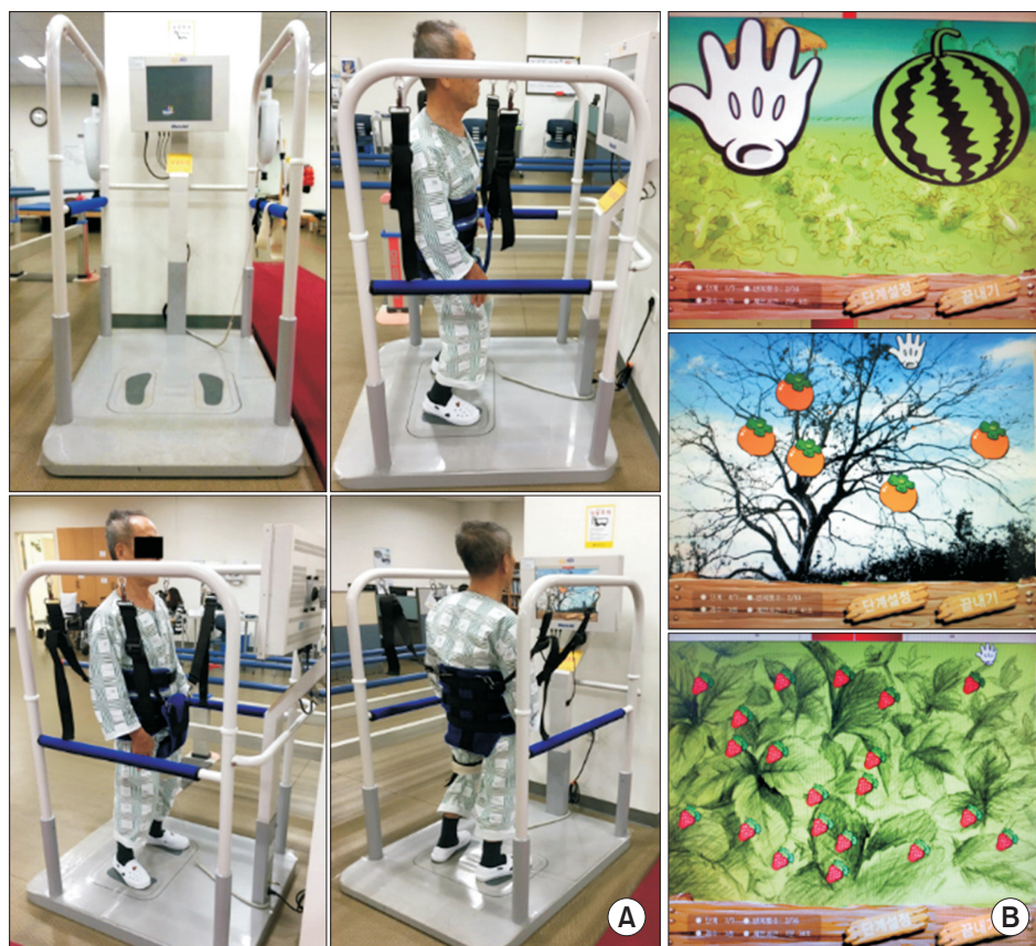
Fig. 2. The balance control trainer (BalPro). (A) The balance control trainer consists of a balance board, a tilting sensor, a computer system, a display screen, and safety bars with a harness. (B) The fruit-harvesting electronic game. The top figure means the easiest level with only one target (fruit) and a large-sized indicator (hand), the middle figure stands for moderate difficulty with several targets (5 fruits) and a middle-sized indicator, and the bottom figure shows the highest level of difficulty with many targets (20 fruits) and a small-sized indicator.
