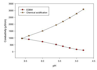
**Figure 1.** Evolution of whey protein isolate (WPI) solution conductivity during chemical and EDBM acidifications.
