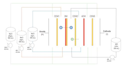
Figure 4. EDBM cell configuration for the electrochemical acidification of whey protein solution.
