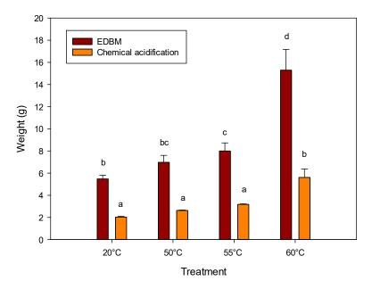
**Figure 2.** Weight of freeze-dried precipitate fractions generated at pH 4.8 after both acidification methods. The results are presented as the means  $\pm$  standard deviation of three independent experiments. The use of different lowercase letters (a, b, c, d) indicate significant statistical differences between data.
