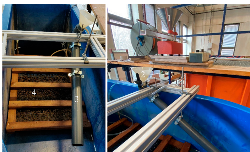
Figure 2. Vibration feeder (1) and anti-air-adherence setup for the particle dosing [funnel with water supply (2) and pipe with 35° inclination (3)]. Furthermore, the flow equilibration is visible (4).
