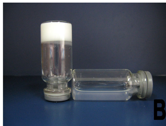
Figure 1 Sol-gel-sol phase transition of PECE hydrogel. A: Sol-gel-sol phase transition diagram. When the concentration was above corresponding critical gel concentration (CGC), the aqueous solution of PECE copolymer undergo a sol-gel-sol transition as the temperature increases. B: Photograph of PECE hydrogel at 10°C (right) and at 37°C (left). At low temperature, the hydrogel is an injectable flowing sol, and forms a non-flowing gel in body temperature.
