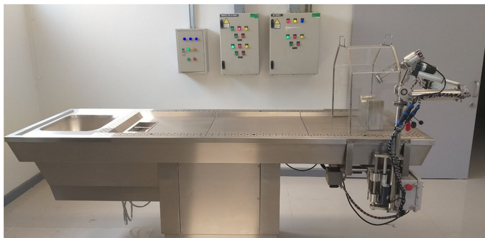
Fig. 4 Prototype of cadaveric skull and tissue cutting manipulator
