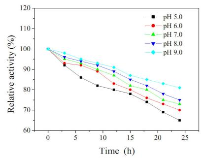
**Figure 4.** The stability of lipase from *Acinetobacter calcoaceticus* 1-7 was measured at pH 5.0-9.0. The lipase was incubated for 24 h at 40 °C in various buffers (0.1 mol/L), sodium acetate buffer (pH 3.0-5.0), sodium phosphate buffer (pH 6.0-8.0), and Gly-NaOH buffer (pH 9.0-10.0). The residual activity was measured with the spectrophotometric assay using p-NPP as a substrate.
