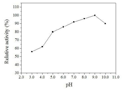
**Figure 3.** Effects of pH on the activity of the lipase. The reaction was determined at 40 °C under different buffers (0.1 mol/L) at various pHs from 3.0 to 10.0, sodium acetate buffer (pH 3.0-5.0), sodium phosphate buffer (pH 6.0-8.0), and Gly-NaOH buffer (pH 9.0-10.0).
