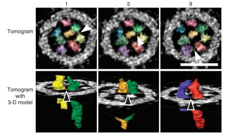
**Figure 2 | Linkages among the eight RNPs in a virion.** Short string-like structures of approximately 2 nm in diameter can be seen between the RNPs (arrowheads). Tomograms, 0.5-nm thick, are shown in the upper row. The 3-D models of two RNPs connected by a string-like structure are shown in the lower row. Virtual slice numbers (1, 5 and 9) of 0.5-nm thick tomograms are given above the tomograms. The colour scheme of the RNPs is the same as that shown in Figure 1b. Scale bar, 50 nm.
