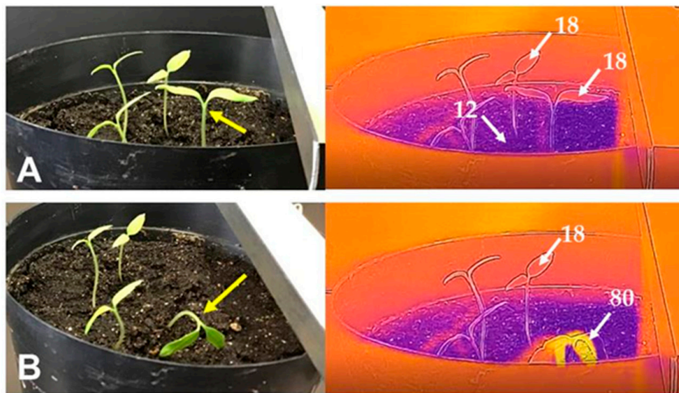
Figure 5. Thermographic detection of arc-discharge-exposed (yellow arrow) and non-exposed shoots of test plants (tomato) sown in pot soil before (A) and after arc-discharge exposure at -12 kV charge (B). Figures in the thermograms represent temperature ( ^{\circ}\text{C} ) measured with a spot temperature meter of a camera. White arrow represents the site of temperature measurement. Note that the arc-discharge-exposed shoot exhibited the highest temperature color (yellow).
