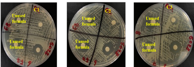
The zone of inhibition for the prepared hand sanitizer and controls against S. hominis 5028
