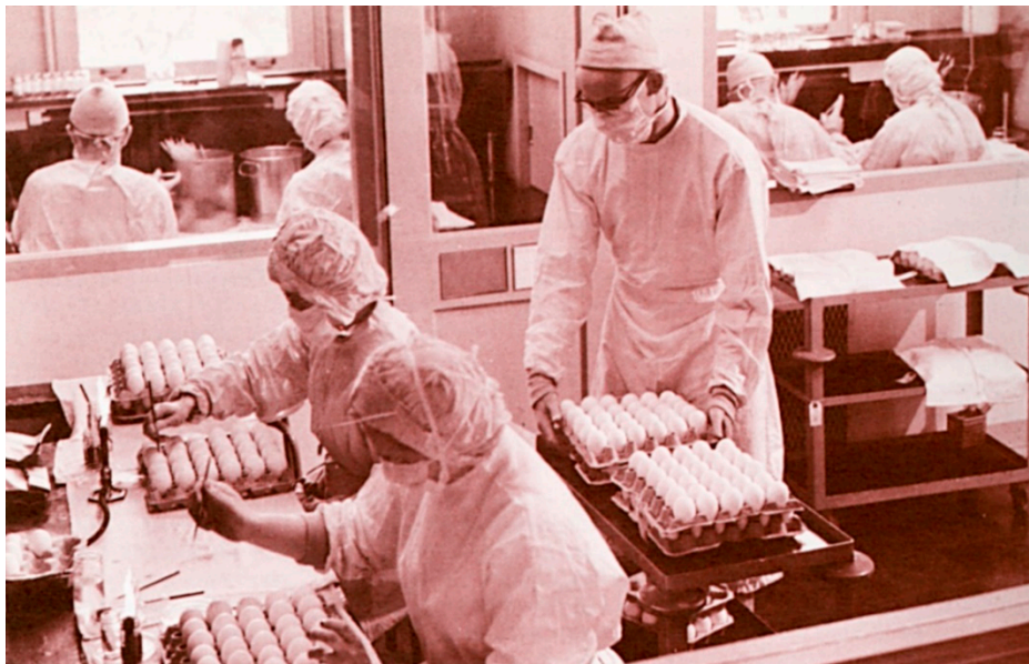
Figure 1. Staff at the New York State Department of Health, Public Health Laboratory (PHL), Division of Laboratories and Research, preparing eggs for inoculation with influenza A virus, to produce vaccines during the 1957–1958 influenza pandemic [9].
