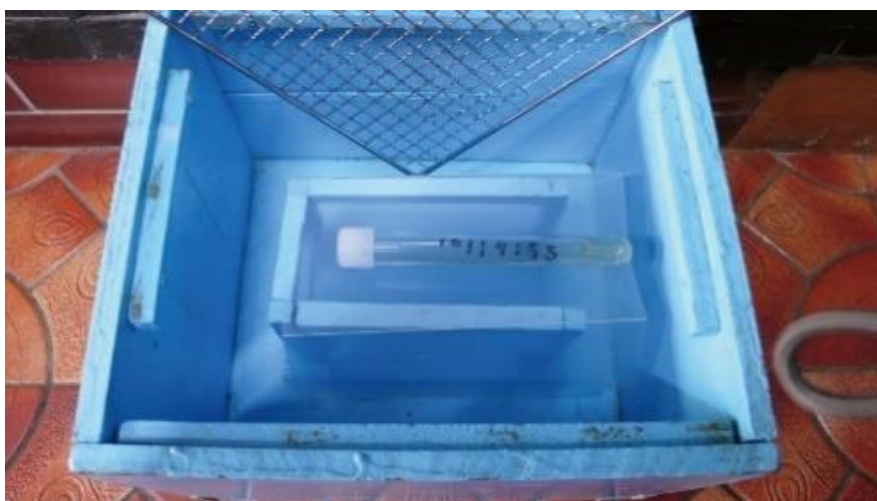
Figure 2. Test Box. The test tube sample with the end cap on was placed in this box.
