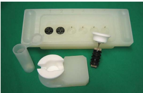
Fig. 2. Sample preparation tools for the REM. The baskets are the same as for the automated LYNX-processor.
