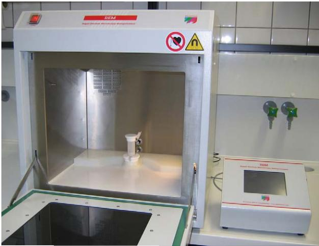
Fig. 1. Milestone rapid electron microscopy (REM) histoprocessor. Note the vial with processed samples placed in a predefined position in the microwave “oven”.
