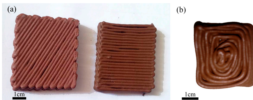
Figure 4. Green samples printed by this method with: (a) appropriate printing conditions; (b) inappropriate printing conditions.
