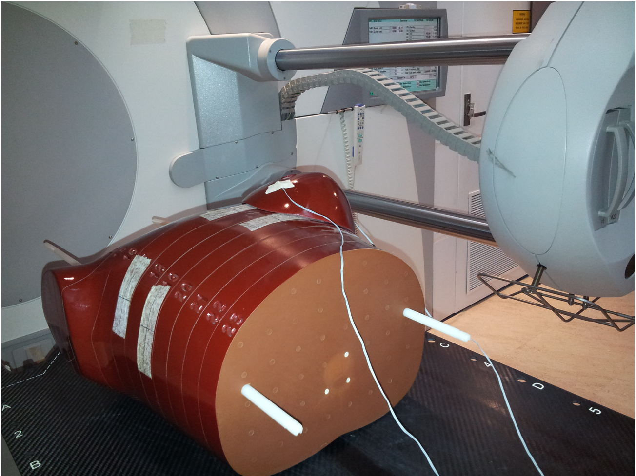
Figure 1: Setup of breast CBCT dose measurement using a female-configured anthropomorphic phantom and MOSFET detectors.
