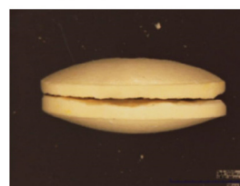
Fig. 5 – Tableting failures: (A) Capping and (B) Binding.
