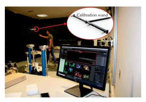
Figure 6. Calibration wand and experiment to determine the location of the markers.
