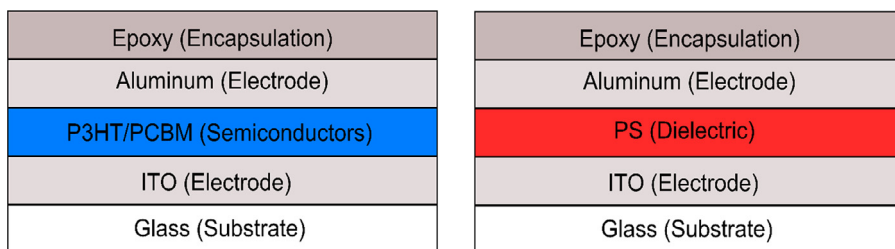
Fig. 1. Schematic diagrams of the BHJ photodiodes (left) and PS control devices (right). The devices are identical except the organic semiconductors are replaced by PS in the control devices. Care was taken to create recipes that produced PS layer thicknesses that matched BHJ semiconductor thicknesses as much as possible.
