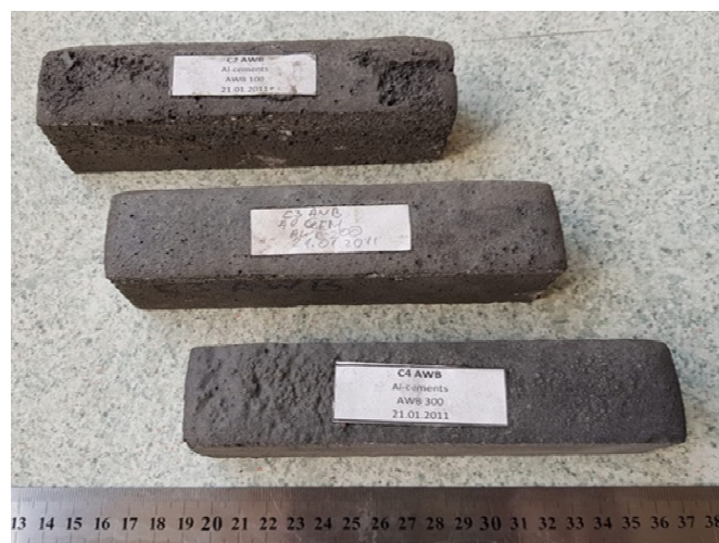
Figure 11. Sample of concrete containing boron 40 × 40 × 160 mm 3 .
