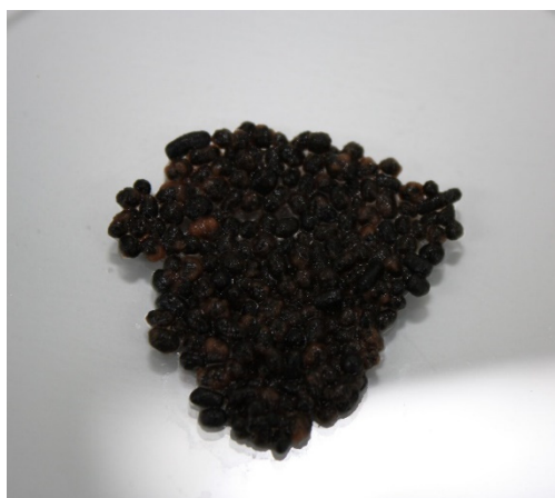
Figure 2. An AOB-loaded activated carbon packing.
