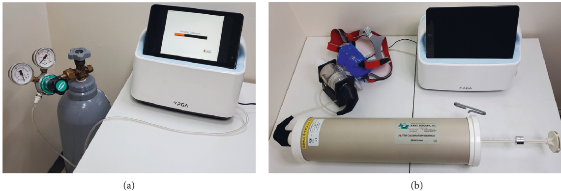
FIGURE 4: Pictures showing the calibration of the developed respiratory gas analyzer. (a) Setup for calibration of the oxygen and carbon dioxide sensors with standard gas containing oxygen levels of 12.33% and carbon dioxide of 2.99%. (b) Setup for calibration of the volume. By using a commercial calibration syringe, calibration was performed with the total volume of 500, 1000, 1500, 2000, 2500, and 3000 ml.
