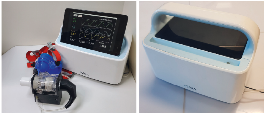
FIGURE 2: The developed portable respiratory gas analyzer, designed for easy measurements. The device is designed to store the tablet PC as well, and the handle serves as a cradle too.
