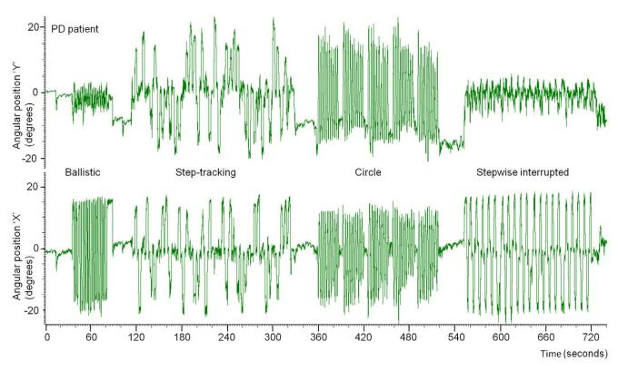
**Figure 3. Single subject kinematic data.** Typical single subject examples of kinematic data for all four movement tasks during scanning (second run of tasks). X-axis: time (in seconds), Y-axis: the angular position (in degrees) of the hand/wrist during movement execution, derived from the two angular position potentiometers (X and Y) integrated in the manipulandum. Top: healthy subject, bottom: PD patient. doi:10.1371/journal.pone.0041042.g003
