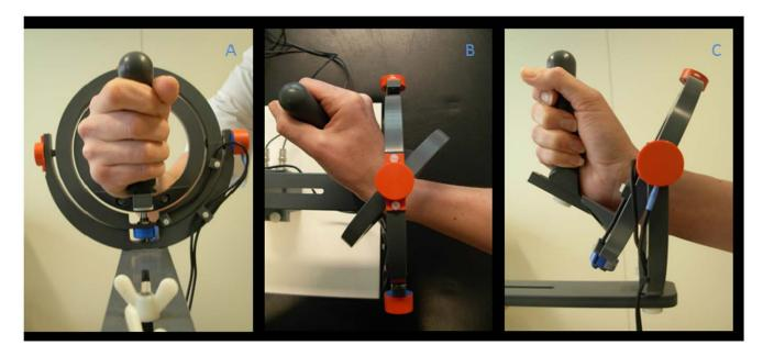
**Figure 1. Photograph of the wrist manipulandum.** The manipulandum consists of two concentric rings moving around perpendicular axes and allowing two degrees of freedom for wrist movement: wrist flexion-extension, ulnar-radial deviation and all combinations thereof. a: (frontal view) neutral position (origin), right hand positioned in a vertical plane holding the grip of the manipulandum; b: (top view) full wrist extension and c: (side view) full radial deviation.
